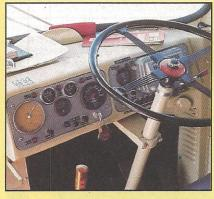
Instrumentation was very basic in those days compared with the luxury coaches of today. The big gauge at left indicated air pressure and was within vision of passengers in the front rows, many of whom thought it registered mph and became quite perturbed when the needle passed 160!
