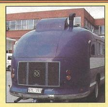
The rounded rear end of Des Feary's Clipper has been fitted with a grille for cooling the rearfacing Perkins V8 engine. The chassis rails were modified to accept the wide cylinder block and manifolds of the big engine.
